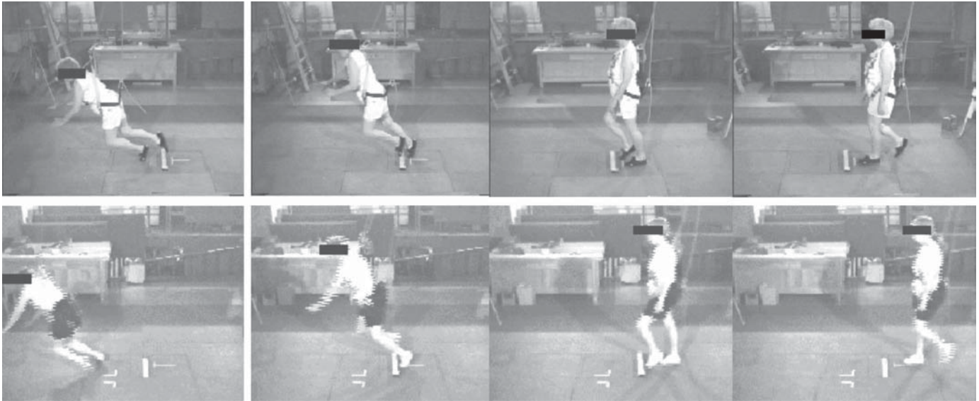
Fig. 2. In the sequences of induced trips, proceeding from right to left, the subjects are protected from falling to the ground by an instrumented harness. During the swing phase of the right leg (sequence at the top) and the left leg (sequence at the bottom), an obstacle rises from the floor and causes the women to trip. (Top) The recovery effort by this older woman was not successful. However, the fall would not expose the hip to impact, making a hip fracture unlikely. (Bottom) The recovery effort by this woman was not successful but, unlike the woman in the top panel, this woman completed a recovery step across the obstacle before “falling.” Note that, in this case, impact on or near the left hip appears imminent. A hip fracture could potentially have resulted were the harness not present.
